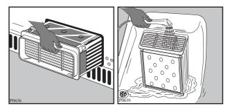
Also clean the outside, removing all fluff. Clean the rubber seal round the porthole door and the seal of the condenser in the inner door with a damp cloth.
